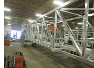
New Ovivo Travelling Bridge Clarifier
